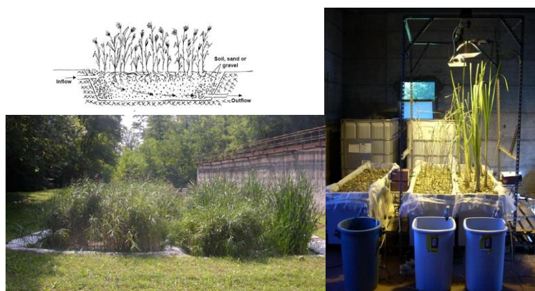
Figure 1.1 – Pictures of the demonstration (left) and of the pilot (right) plants and scheme of a horizontal subsurface flow system)
