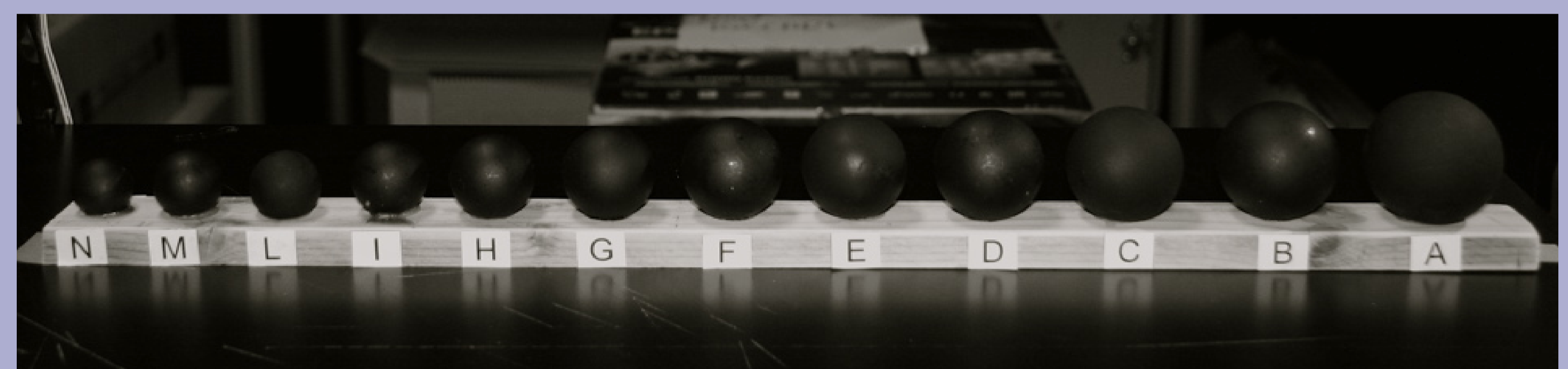
Visual scale (60 cm) made of 12 metallic spheres painted matt black: 2.2, 2.5, 2.7, 2.9, 3.1, 3.5, 3.8, 3.9, 4.1, 4.3, 4.5, and 4.7 cm
