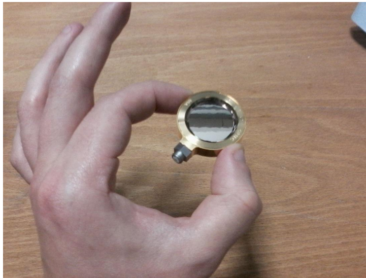
Figure 3.4: Picture of a 500 \mu\text{m} thick silicon detector.
