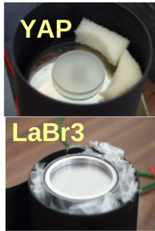
Figure 3.9: of a 2 mm thick YAP and LaBr 3 scintillators.
