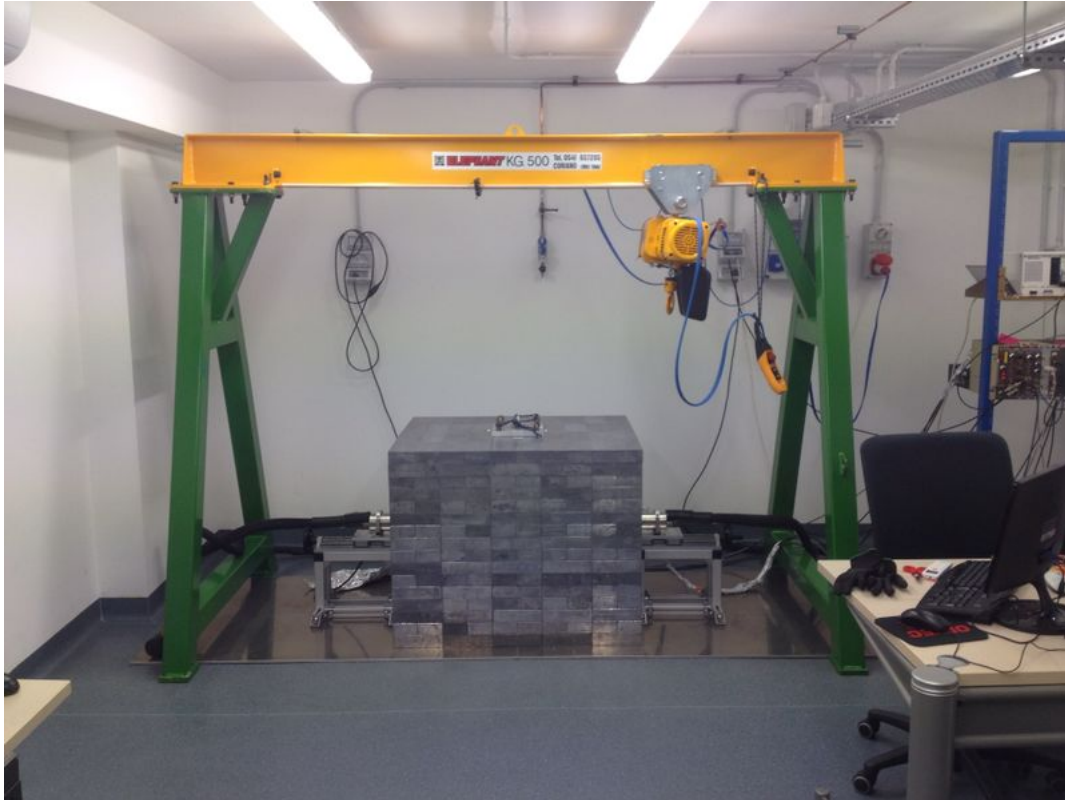
Figure 4.15: Lead shielding and the winch-crane system
