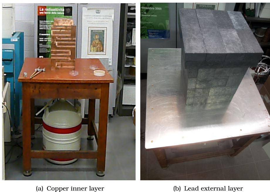
Figure 6.5: The BEGe preliminary shielding
