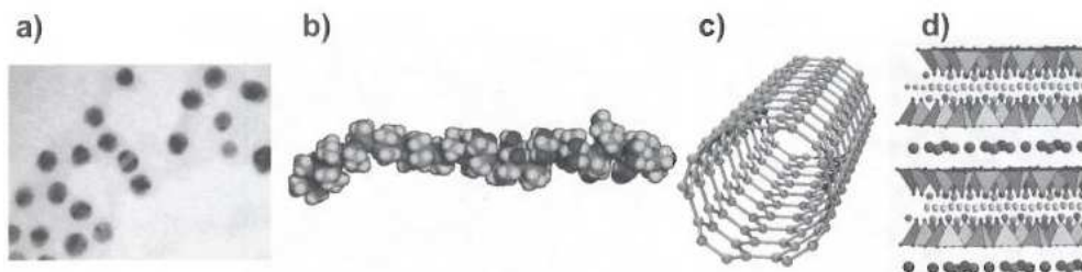
Fig. 1.3 Some different inorganic building blocks used in nanocomposites materials: a)nanoparticles, b) macromolecules, c)nanotubes, d)layered materials
