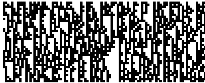
Figure 36: The space-time diagram of the probabilistic xor CA of Example 15.1.1. A black (resp., white) box stands for a 1 (resp., 0). \mu is the uniform measure over \{0, 1\}^{\mathbb{Z}} . Time goes downward.
