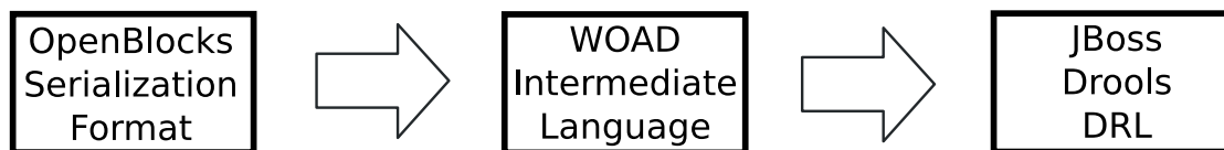
Figure 7.5.: The translation process from OpenBlocks serialization format to DRL
