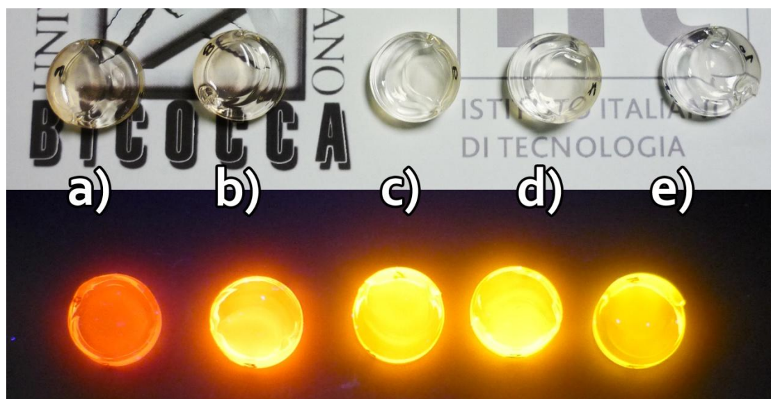
Figure 7.8 Bulk polymer nanocomposites made of PMMA and a) \text{Cu}_{0.7}\text{In}_{0.77}\text{Zn}_{0.85}\text{S}_2 b) \text{Cu}_{0.42}\text{In}_{0.71}\text{Zn}_{0.64}\text{S}_2 c) \text{Cu}_{0.26}\text{In}_{0.8}\text{Zn}_{0.72}\text{S}_2 d) \text{Cu}_{0.18}\text{In}_{0.65}\text{Zn}_{0.52}\text{S}_2 and e) \text{Cu}_{0.13}\text{In}_{0.74}\text{Zn}_{0.59}\text{S}_2 nanocrystals. In the upper image the samples are shown under sunlight. In the lower image the nanocomposites were illuminated with an UV lamp ( \lambda=450\text{nm} ). The diameter of every single thick disk is 2.5cm.
