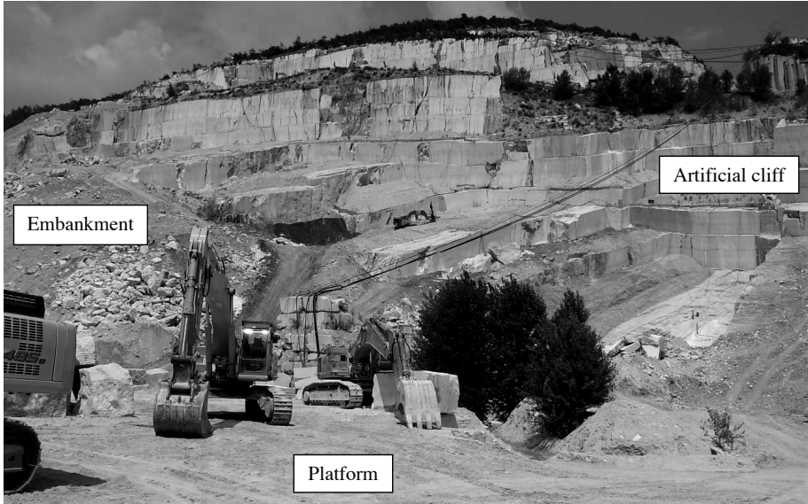
Fig. 1.2 Main geomorphological surfaces on quarries: artificial cliffs, embankments and platforms; Quarry “Coop. Operai Cavatori del Botticino” (ATE 1 3/2), Botticino (Lombardy, Italy)
