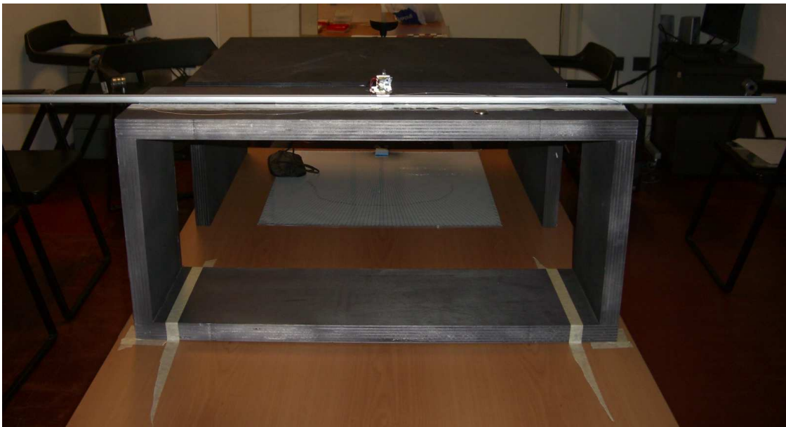
Figure 11. Box used in the Visual and Visual-proprioceptive tests. On the table, the goniometry board to record the error of the pointing movement
