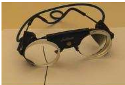
Fig. 3 - Rightward-shifting prism inducing a 10° lateral shift of the visual image
