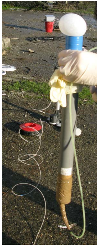
Figure 53: detail of the tool used to tracer injection
