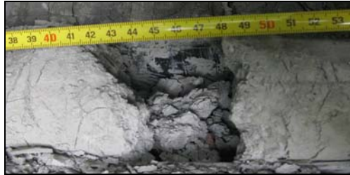
Figure 34: fracture with evidences of gypsum dissolution at 16.50 m BGS from the extracted S16 core.
