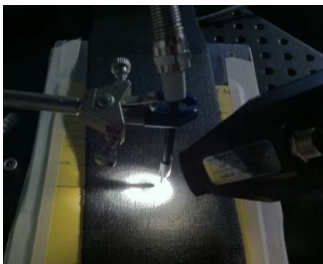
Figure 6.5. FORS setup used to collect the spectra in reflectance of the uncoated and coated black paint.
