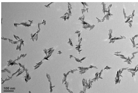
Figure 4.1. TEM of TiO 2 rutile nanoparticles.
