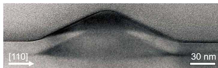
Figure 3.3: TEM image of two stacked SiGe islands, from [83].
