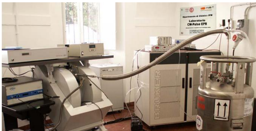
Figure 2.5. ELEXYS 580 Bruker spectrometer used in the group of Prof. Elio Giamello at the University of Turin.
