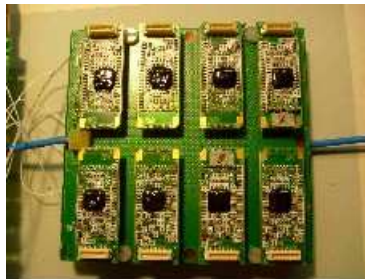
Figure 5.4: Readout board with 8 CARIOCA chips.
