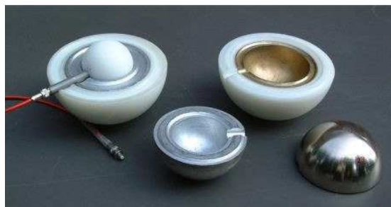
Figure 1. Bonner spheres with metallic inserts.
