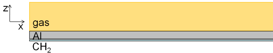
Figure 5.6: A thick Al cathode (grey) is used to suppress detection of neutrons with oblique incidence. Only one of the four protons in the figure can cross the Al layer and produce a discharge in the GEM gas.
