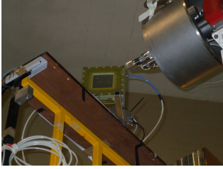
Figure 5. Analog nGEM prototype installed in the FNG bunker close to the neutron gun.
