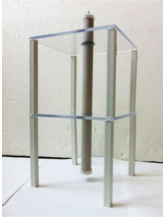
Figure 5.9: The gradient index lens, with wax coating and support adjustable in height.
