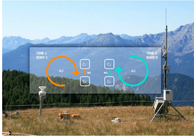
Figure 2.2: Exemplification of eddy flux at a single point (from Burba and Anderson (2010) modified). At a given instant (time 1), eddy number 1 moves air parcel c_1 downward with the speed w_1 . At the next instant (time 2) at the same point, eddy number 2 moves air parcel c_2 upward with speed w_2 . Each air parcel has its own characteristics, such as gas concentration, temperature, humidity, etc. the eddy covariance samples how many molecules of gas go down to the biosphere with downward wind at time 1 and how many go up to the atmosphere with upward wind in time 2.
