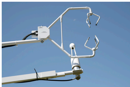
Figure 2.3: Example of an Eddy Covariance installation, composed by a 3-D sonic anemometer (CSAT3, Campbell Scientific, Inc.) and an open-path IRGA (LI-7500, LI-COR, Inc., Lincoln, NE, USA)
