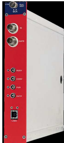
FIGURE 5.13: CAEN MCA used to perform the acquisition with event time information.
