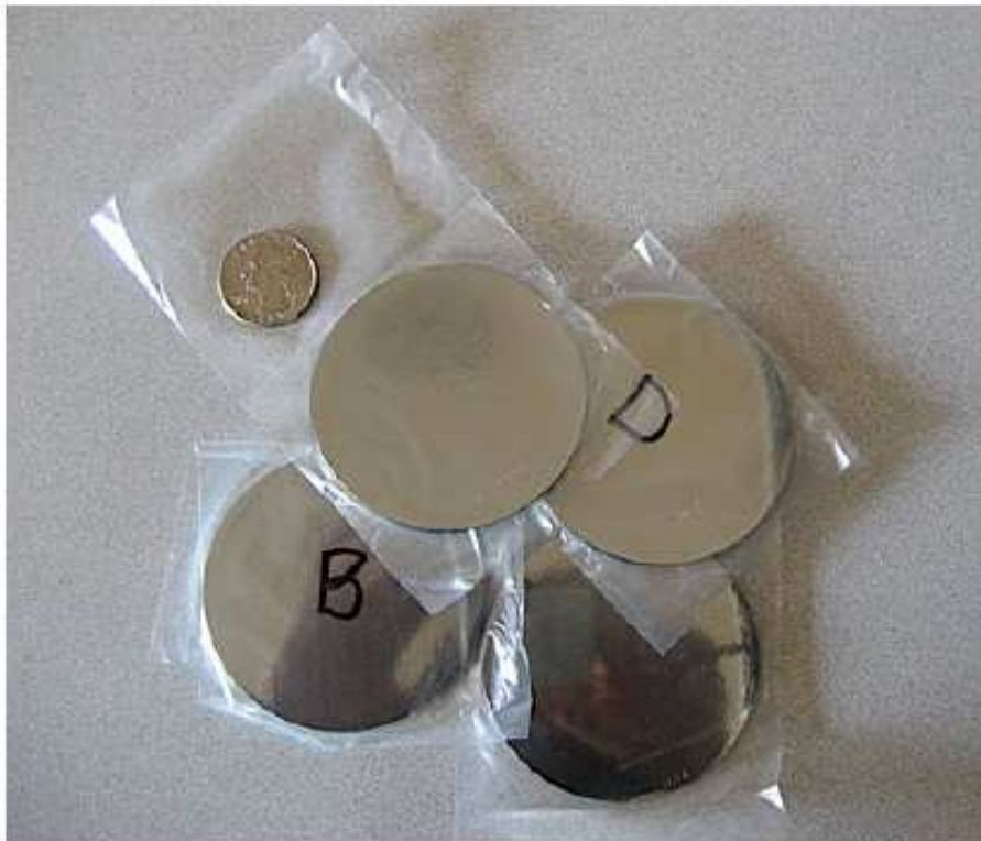
FIGURE 4.2: Germanium wafers used to make NTD Ge thermistors.
