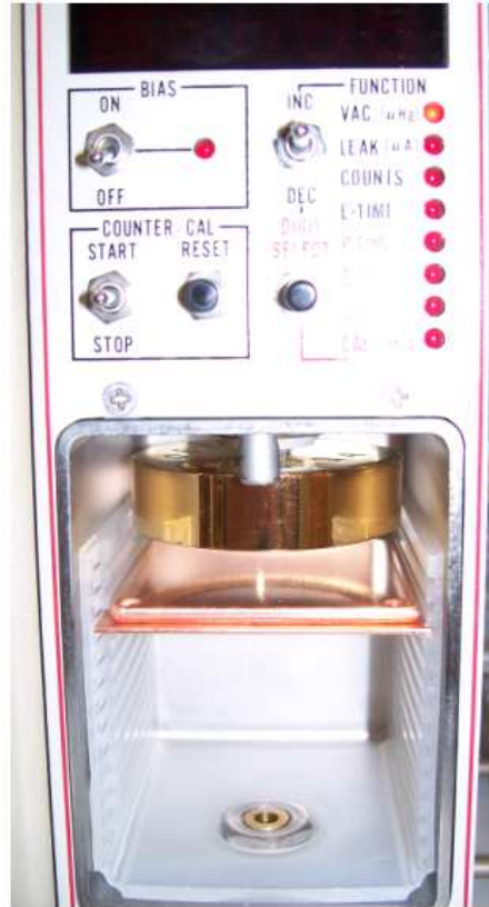
FIGURE 5.6: A picture of a vacuum chamber where the SBD's are operated. From the top: on the left there is the bias control, on the right there are some status control leds (to check leak current as well as vacuum level...). In the center there is the chamber with a silicon detector inside faced to a copper sample.
