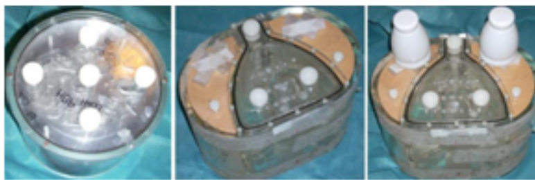
Figure 2.1: The anthropomorphic phantoms: the Hoffman 3D brain phantom (left), the thorax phantom (center), the breast phantom (right)
