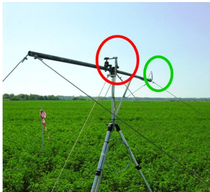
Figure 3.7: Typical setup of MRI installation in field: the tripod supports the ends of the optical channels. The red circle evidences the cosine corrector receptor, the green one indicates the end of the down-looking channels (bare fibers).
