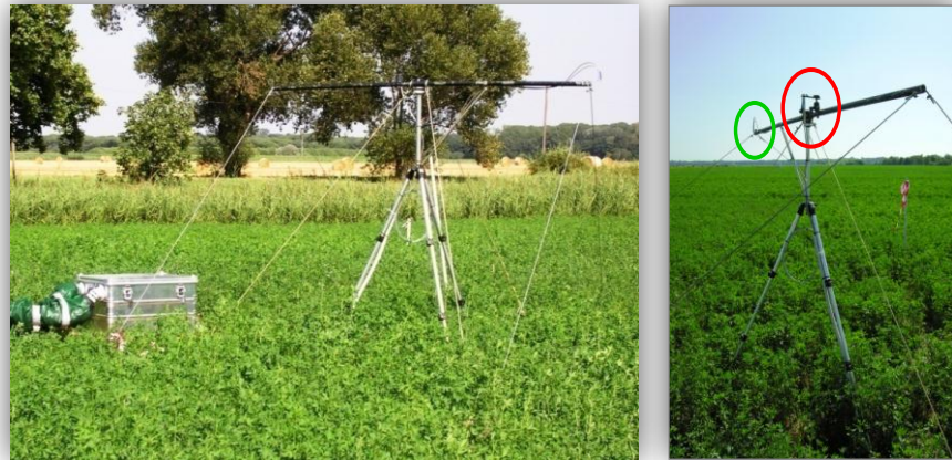
Figure 5.10: Multiplexer Radiometer Irradiometer MRI operated in the framework of the Sen3Exp field campaign at the alfalfa measurement site. On the left the MRI automatic system, the thermally-regulated box hosts the optical system and electronics. On the right detail of the terminations of the instrument optical system, red and green circles highlight the uplooking (cosine receptor) and downlooking (25° FOV) foreoptics, respectively.
