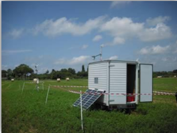
Figure 5.11: Mobile micrometeorological station installed at the alfalfa experimental field.
