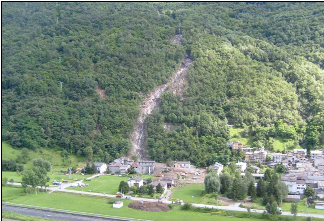
Fig. 10.4 – Aerial photograph showing lower part of the Selvetta debris flow. Photo F. Luino.
