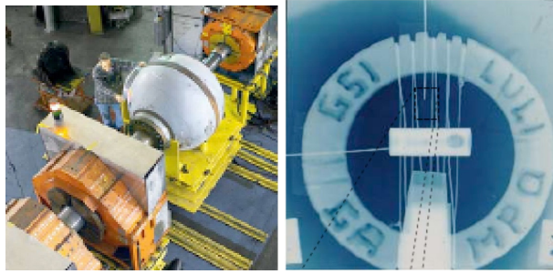
Fig. 4: Left) a 3-ton steel vessel used to confine the explosion involved in proton-radiography experiments is flanked by large orange electromagnets focusing the protons to produce sharp radiographs at Los Alamos. Right) proton radiography with \sim 8 MeV laser-generated protons by M. Roth et al. at LULI showing the ability to discriminate different thicknesses and densities
