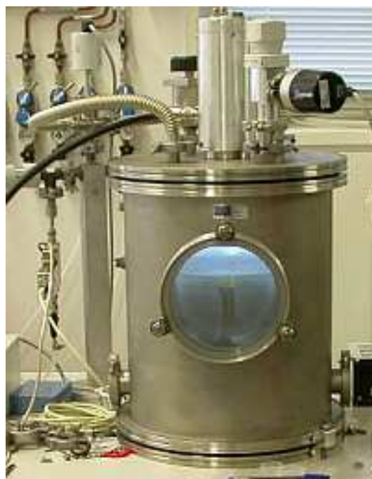
Figure 3.2: Picture of the reactor A running. Inside the chamber the typical azure glow of argon gas discharge is visible.
