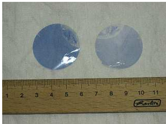
Figure 3.11: ppAAc disks after the immersion in a solution of THA
