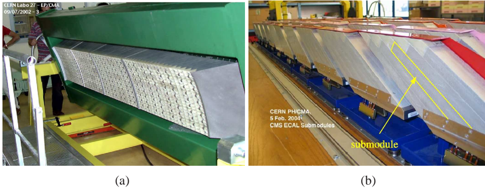
Figure 1.12.: (a) Photograph of the supermodule, showing the single modules. Each supermodule is composed of 4 modules. (b) Submodule of the ECAL. Each submodule consists of 10 crystals in a glass-fibre alveola structure.
