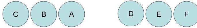
Figure 5.5: A scheme of the input FOV of the spectrometer. This coincides with the telescope focal plane.
