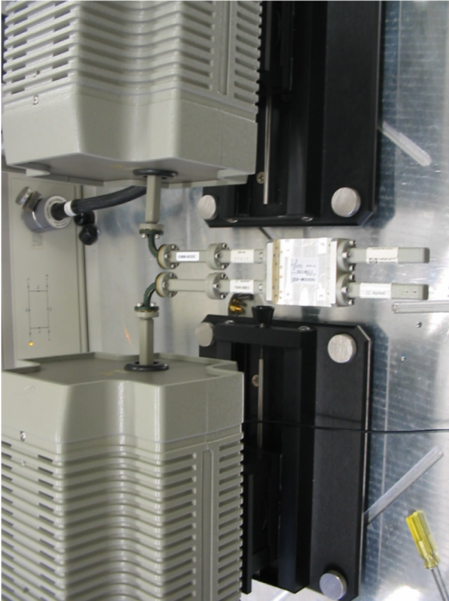
Figure A.2: Picture of the experimental setup for MVNA hybrid ring measurements.
