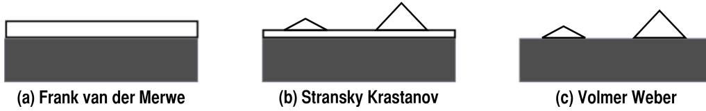
FIGURE 2.1: Heteroepitaxial growth modes. (a) Layer by layer, or Frank van der Merwe (FM) growth. (b) 3D island formation on top of thin wetting layer, or Stransky Krastanov (SK) growth. (c) 3D island formation on top of the substrate surface, or Volmer Weber (VW) growth mode.
