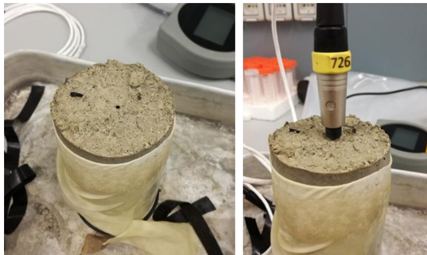
Figure 2.9: Frozen soil specimen of dimension according with ASTM D5334-08 with needle probe of Thermtest Portable TLS-100 during thermal conductivity measurement.
