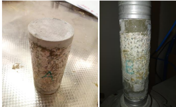
Figure 2.4: Treated soil specimen equipped with specific cement plinth to ensure a flat base.
