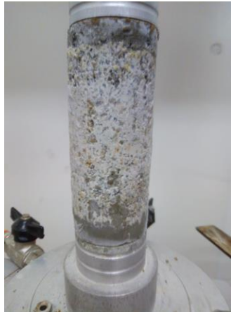
Figure 2.31: Triaxial compression tests results of TS sample at -10 °C.
