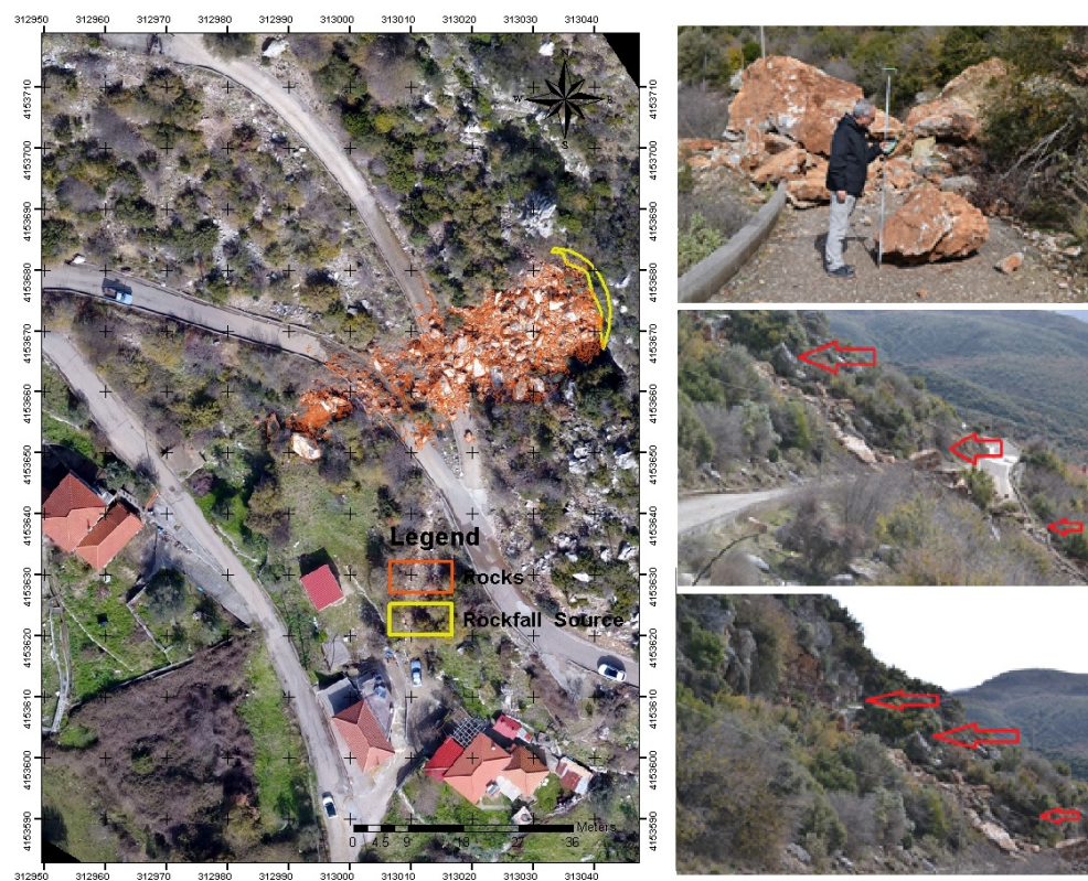
Figure 2. Pictures of the rockfall in the Myloi region illustrate the final position of rock blocks. Red arrows indicate the final positions of the rock masses at the conclusion of the rockfall event.
