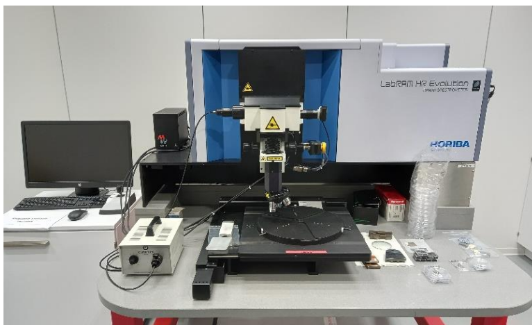
Figure 2.11: Raman spectrometer used for the characterization of the phase composition in UFP samples.
