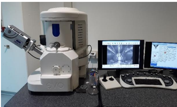
Figure 2.5: EVO MA10 Scanning Electron Microscope used for the morphological and chemical analysis. The EDXS detector can be observed on the left side (front image).
