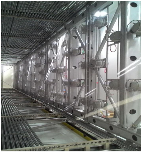
Fig. 4 The new ICARUS PMTs mounted behind the wires of one TPC
