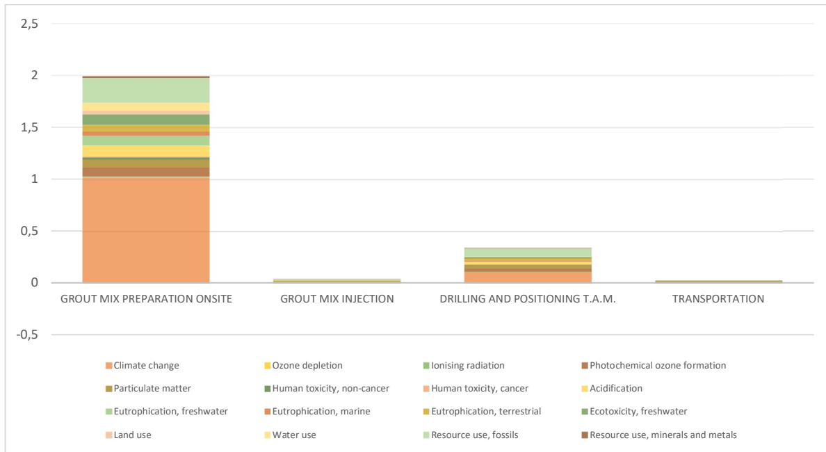
Fig. 8-9, Permeation Grouting technique: impacts, single point view.
