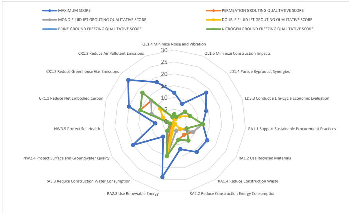
Fig. 7-6, First Phase Output: The sustainability performance of the five ground improvement techniques under the Envision and the DNSH scoring. A comparison through the radar diagram view.
