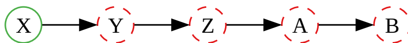
■ Figure A1 Graph \mathcal{G} of a CTBN model consisting of a chain of five processes.
