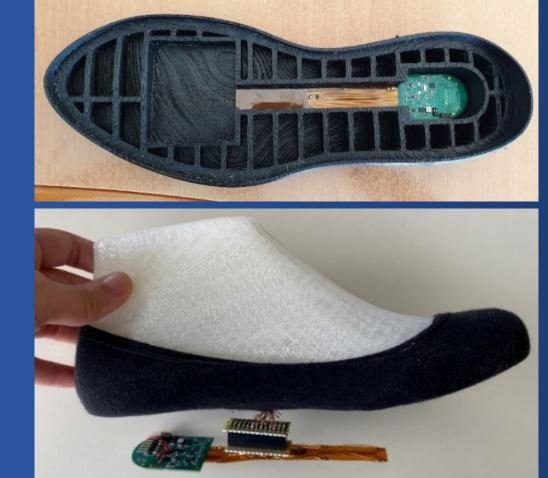
In the electret case a 3D TPU flexible arc structure allows to cyclically vary the electrostatic coupling strength on a multistrip plane, and then the system capacitance.
