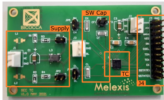
Figure 5.2: Picture of the PCB for testing designed for the TC1
