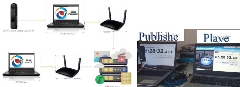
Figure 5 - Test setup for end-to-end latency measurement.
