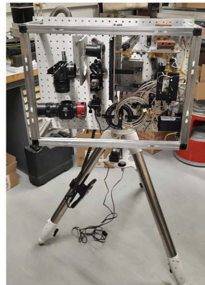
Figure 1. Left: mechanical drawings of the COSMOCal box containing the: microwave source components (right) and the optical system (left). Right: first assembled version.
