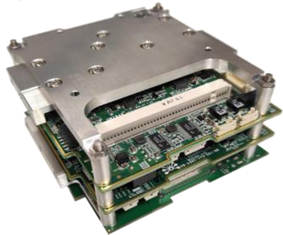
Figure 8. Unibap's iX5-100 processor unit flown aboard D-Orbit's ION SCV-4 satellite
