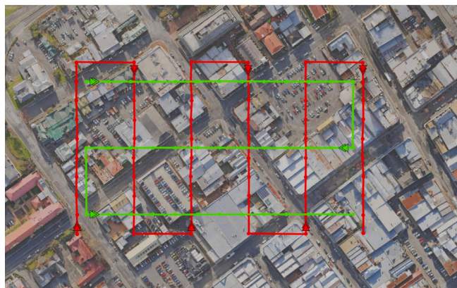
Fig. 5. Camera paths on the ENRICH-Aerial dataset. In red the path followed by the first nadir and oblique cameras, in green the path followed by the second nadir camera. (For interpretation of the references to color in this figure legend, the reader is referred to the web version of this article.)
