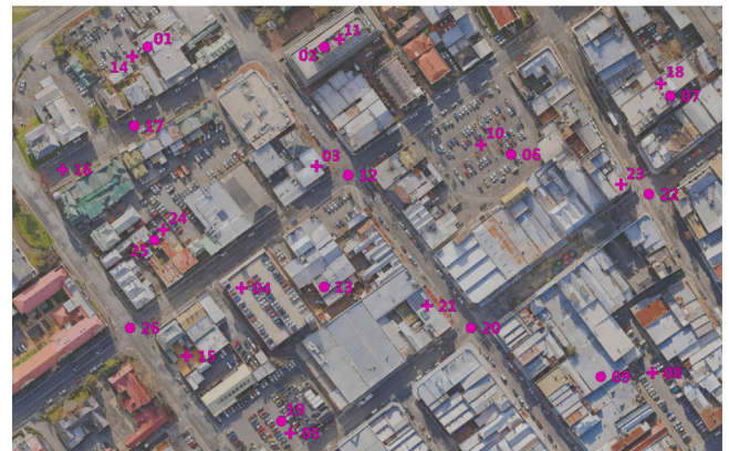
Fig. 2. Orthographic view of the GCP placement on the ENRICH-Aerial dataset. Cross and round shapes as in Fig. 3.
