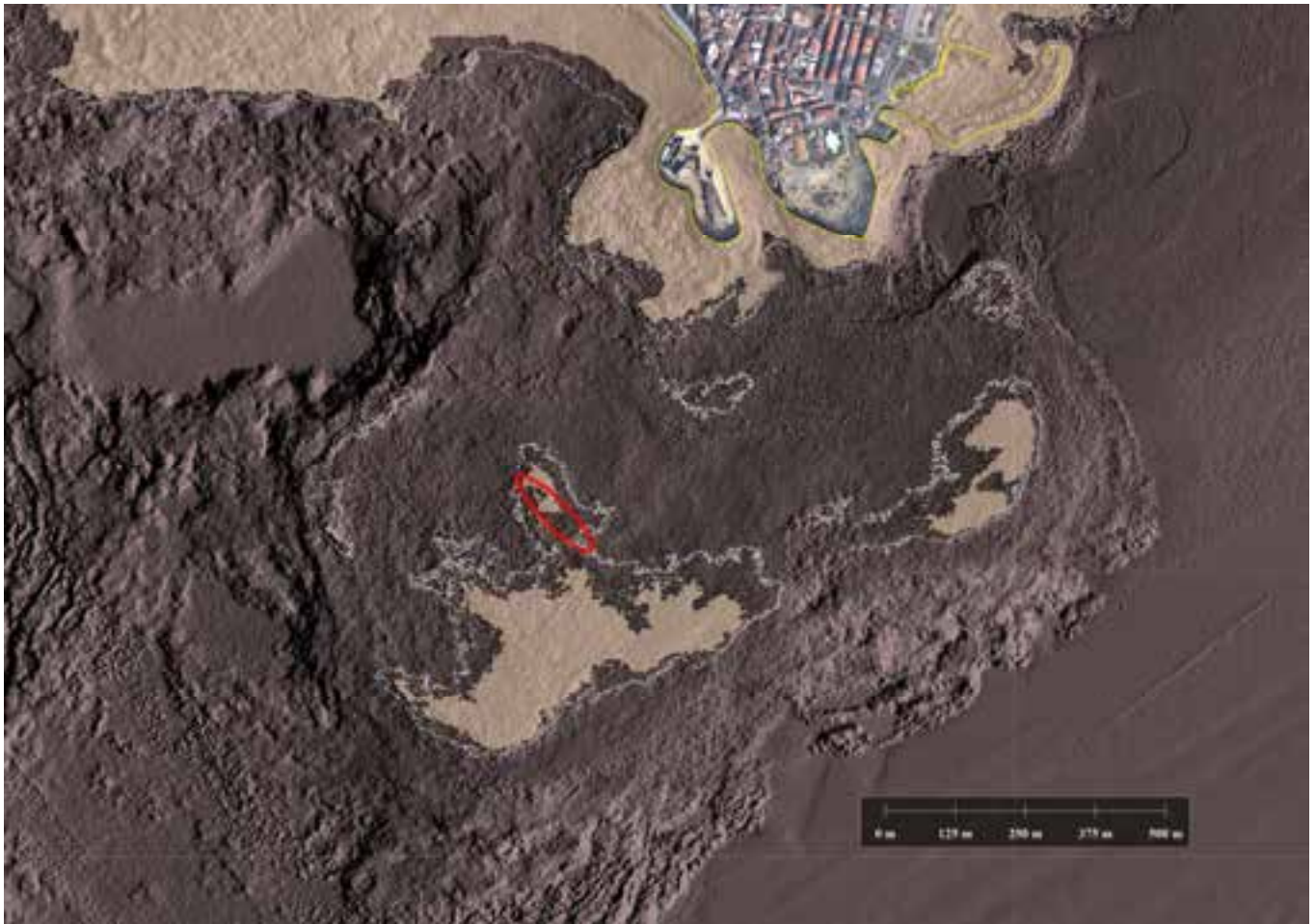
Figure 26. The DTM from MBES with the outcomes of the paleo-geographic simulation of the area with a sea level lower than 9.5 m, considering both the local uplift and sliding (for details, see Geological setting). The white isobath indicates a fixed isoline created with GlobalMapper and rigidly placed at -9.5 m, while the light beige fill indicates the result of an algorithm that hypothesises the water drainage on a 3D surface. In this last model, we used the “Simulate Water Level Rise/Flooding” of Global Mapper. To improve the readability of the plan, we have excluded the closed isolines with a perimeter of less than 300 m. The red ellipse roughly outlines the localisation of the extrabasinal materials, as shown in Figure 19. Simulation elab. by F. Mauri.
