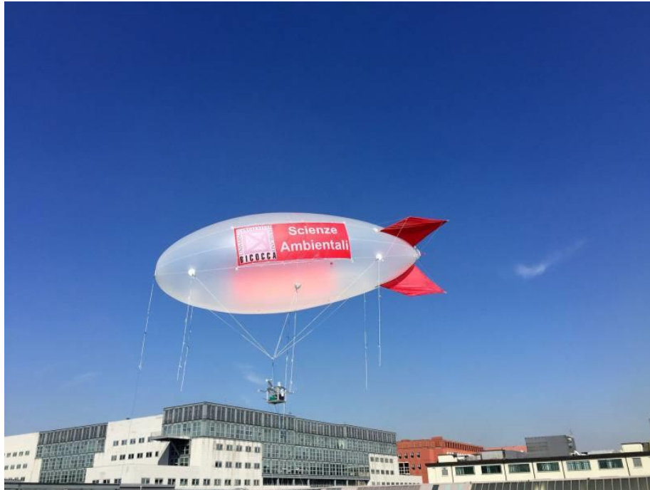
Figure 1: Helium-filled tethered balloon (14 m long and diameter of 3 m) with the equipped Plexiglas platform.
