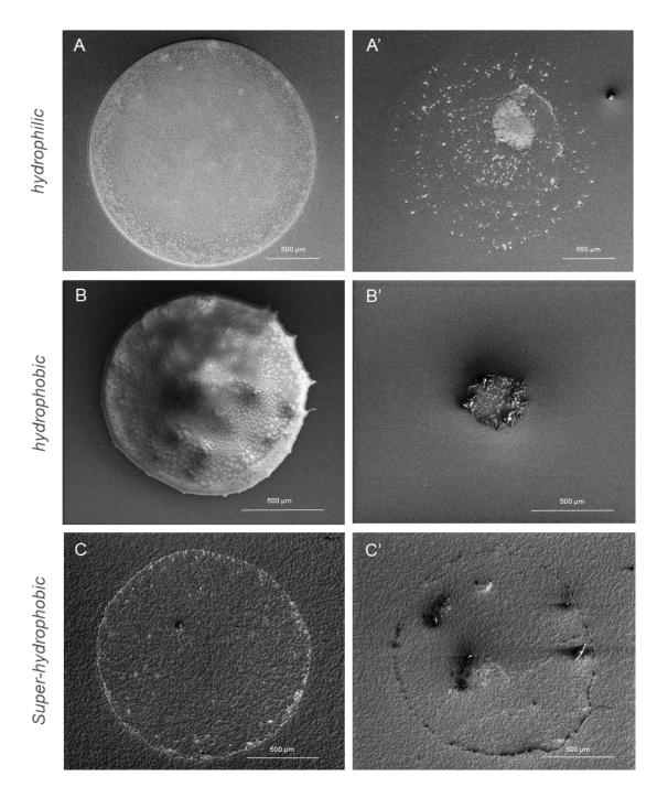
**Figure S6.6.** Scanning electron micrographs of processed sample  $(1 \ \mu L)$  of on hydrophilic (panel A), hydrophobic (panel B), and super-hydrophobic surface (panel C) after digestion (A, B, C) and the following purification step (A', B', C'). This comparison illustrates the influence of the hydrophobic properties of the surface and the impact of both processes on the characteristics of the sample and highlights the improvements achieved with purification.
