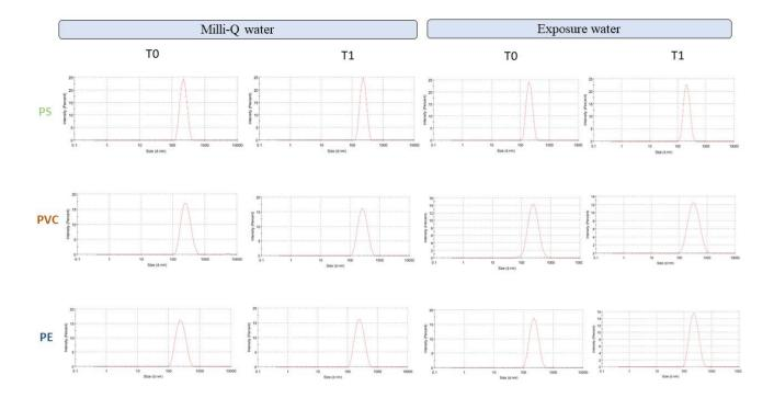
Figure S3.2 DLS intensity measurement of PS-NPs, PVC-NPs and PE-NPs at T0 and T1 in both Milli-Q and exposure waters.
