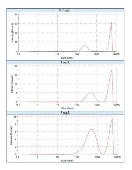
Figure S5.1. DLS measurements of hydrodynamic size expressed as intensity distributions of the three investigated NMFs concentrations (0.2 mg/L, 1 mg/L and 5 mg/L) in the exposure test water
