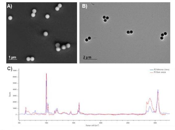
**Figure S6.5.** Characterization of PS-NPs 500 nm by SEM (A), TEM (B), and RAMAN (C) after digestion steps. Raman spectra: blue line = PS reference spectra, red line = PS after extraction protocol.
