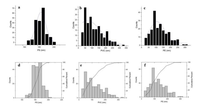
Figure S3.3: Histograms in the top row report the MinFeret (nm) size distribution and relative Gauss fit for PS-NPs (a), PVC-NPs (b), and PE-NPs (c), calculated through TEM measurements. The lower row reports the corresponding cumulative percent curves for PS-NPs (d), PVC-NPS (e), and PE-NPs (f).
