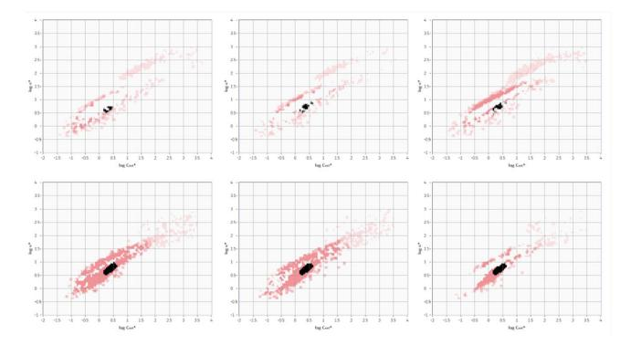
**Figure S6.4.** SPES raw data illustrating the PS500 spiked sample after subtracting the matrix contribution. The data is presented for triplicate samples spiked with polystyrene at  $10^7$  particles/mL (first line) and  $10^9$  particles/mL (second line).
