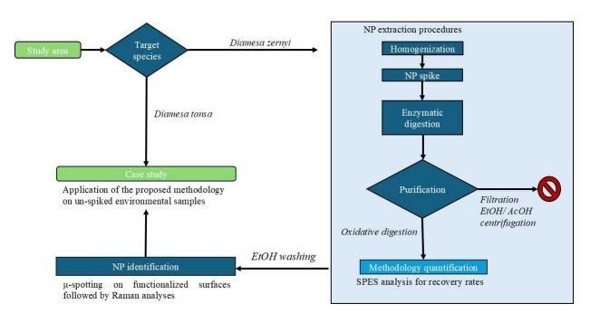
**Figure 6.1.** Analytical workflow representing the different steps performed in the development of an analytical method for the detection of nanoplastics in biological samples.
