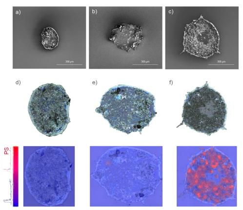
**Figure 6.3.** Scanning electron micrographs and white light montage with relative mapping with Raman images overlay of control (a, d), spike  $10^7$  particles/mL (b, e) and spike  $10^9$  particles/mL (c,f). The red dots in the Raman images (bottom) highlight if the PS is present in the sample.
