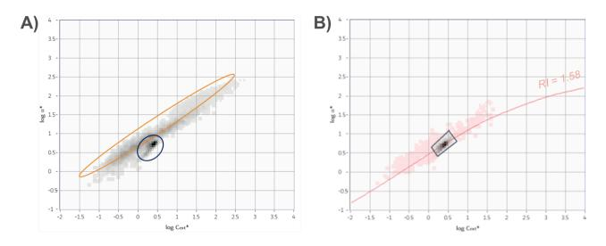
**Figure S6.1.** SPES raw data of a sample with PS500 spikes (left). In the 2D histogram, the single population of PS500 (RI = 1.58) in the heterogeneous sample can be selected (right).
