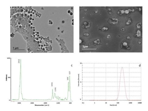
Figure S4.2. Transmission electron microscopy (a), scanning electron microscopy (b), Raman spectra (c), and DLS intensity measurement (d) of PVC-NPs. The numbers in the Raman spectra specify the peaks used to identify PVC.
