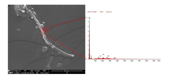
Figure. S5.3. Detail of a SEM image of a single microfiber (on the left) and its elemental composition investigated through energy dispersive X-ray spectroscopy (EDS) analyses. Gold (Au) and palladium (Pd) signals derived from the sample preparation, while oxygen (O) is from the atmosphere of the sample chamber. The spectrum of the samples exhibits C as expected for polypropylene.
