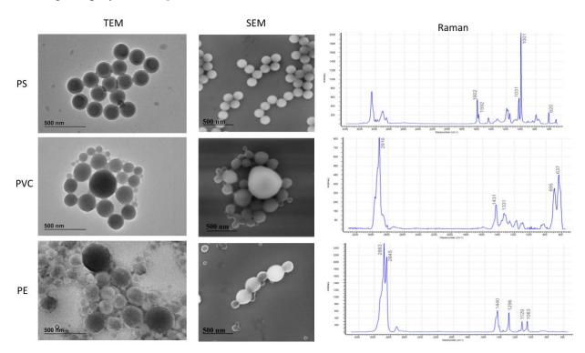
Fig. 3.1. Transmission electron microscopy (TEM), scanning electron microscopy (SEM) and Raman spectra of PS-NPs, PVC-NPs, and PE-NPs. The numbers in the Raman spectra specify the precise peaks utilized to identify PS, PVC, and PE polymers.
