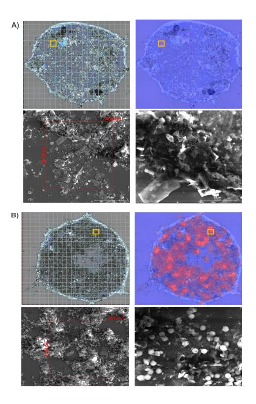
**Figure S6.8.** Above are the white light montage images of the entire sample area (step size 20  $\mu$ m) alongside the corresponding Raman image. The yellow square highlights an example of a scanned area (20 x 20  $\mu$ m) where polystyrene (PS) was detected. In the lower part of the figure, the corresponding scanning electron micrographs of that area confirm the variation in particle number between regions of low (A) and high (B) PS spiked concentration.
