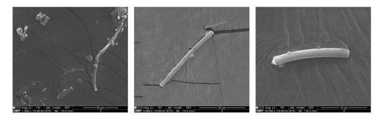
Figure. S5.2. Scanning electron microscopy (SEM) of the photodegraded NMFs.
