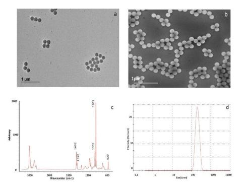
Figure S4.1. Transmission electron microscopy (a), scanning electron microscopy (b), Raman spectra (c), and DLS intensity measurement (d) of PS-NPs. The numbers in the Raman spectra specify the peaks used to identify PS.
