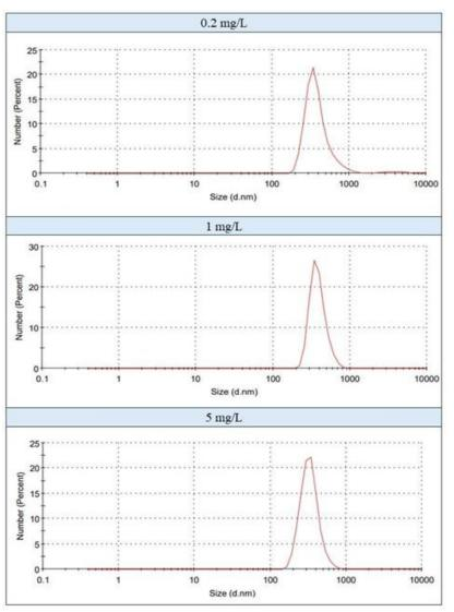
Fig. 5.1. DLS measurements of hydrodynamic size expressed as number distributions of the three investigated NMF concentrations (0.2 mg/L, 1 mg/L and 5 mg/L) in the exposure test water.
