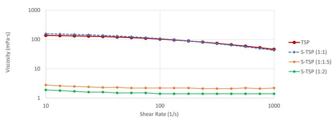
Fig. 3 Viscosity of TSP and S-TSP samples at 20°C obtained by Modular Compact Rheometer (Double Gap)
