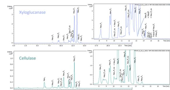
Fig. 7 HILIC/ESI-MS of TSP hydrolyzed with Xyloglucanase and Cellulase (P - pentose, Hex - Glc o Gal)
