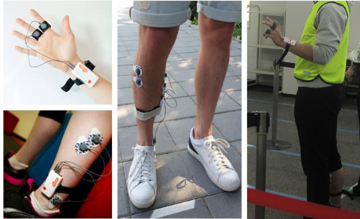
Figure 20: Figure showing the sensors used throughout the experiment. The two images to the left show the GSR and PPG sensor (up) and the EMG sensor (down), while the central image and the right one show how the participants wore those same sensors during the experimental sessions.
