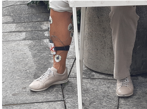
(b) Image depicting how participants wore the EMG Shimmer sensor during the experiment.
