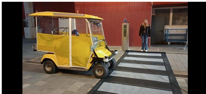
Figure 2: The vehicle approaching the crosswalk. In this picture, the vehicle is in autonomous mode, with an operator on the passenger seat, wearing a hat occluding eye-contact with the pedestrian. Nobody is sitting at the steering wheel.
