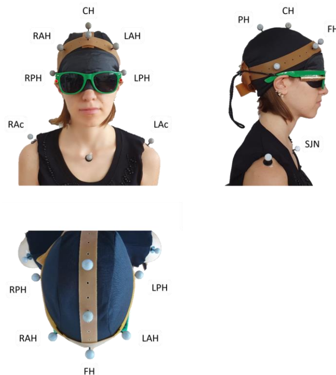
Figure 1. Personalised marker model (rubber “crown” set up). FH: frontal head marker; CH: central head marker; PH: posterior head marker; RAH and LAH: right and left anterior head markers; RPH and LPH: right and left posterior head markers; RAc and LAc: right and left acromion; SJN: sternum jugular notch. Two bullet-like laser pointers, projecting a red light beam, are fixed on a pair of glasses tightened posteriorly. The participant wears a sleeping mask to prevent visual cues. The subject’s gaze points downwards in the bottom panel (horizontal view) and rightwards in the right panel (sagittal view). The subject’s spatial orientation can also be inferred by looking at the corresponding marker labels.
