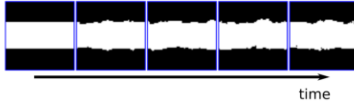
Figure 63: Example of a KMC simulation results for the evolution of a simple stripe under edge diffusion. As time progresses, the roughness of the interface increases.
