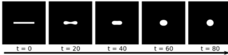
Figure 39: Example of an evolution by surface diffusion of a simple rod-like domain as obtained through FEM solver. The final state is circular, consistent with the sharp interface model. t is measured in terms of time separation between training set snapshots.
