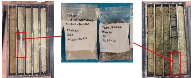
Fig 6.34 Panaro sand tested with cyclic simple shear test, in the box (Bicocca university) and in the bags (Dundee University)
