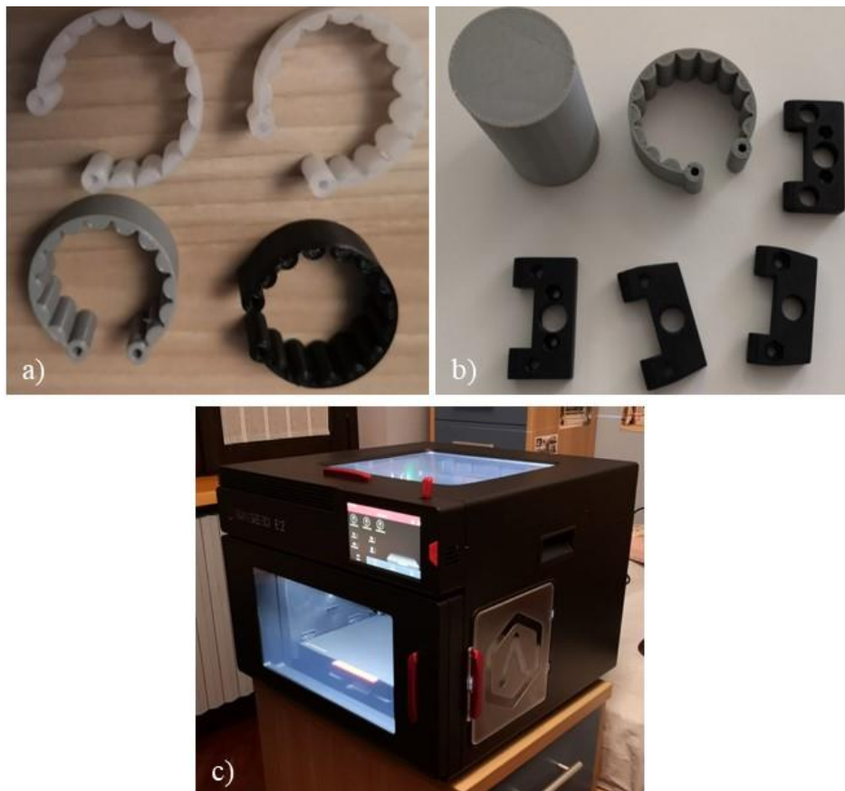
Fig 8.5 Development of new on sample support: a) Radial chain made of different material; b) Rigid sample used to test different chain along with support for transducer; c) 3D printer used to prepare the chain and support
