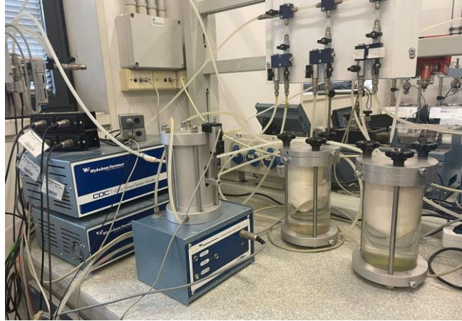
Figure 6.1 Pressure and volume change control: air-water bladder and automatic volume change apparatus
