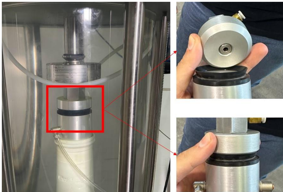
Fig 8.11 Vacuum system with suction cup to allow extension of the sample during the test
