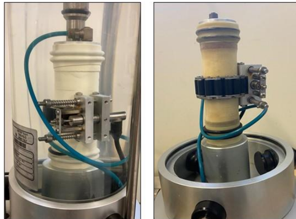
Fig 8.4 On sample radial transducer, prototype developed in 2021
