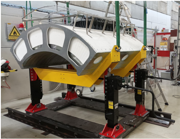
Fig. 17 The ENUBET demonstrator in the CERN T9 beamline. The white layer between the inner part of the detector and the SiPM electronics is the borated polyethylene shielding. During the test, only 20% of the detector (length: 80 cm, 18° coverage in the azimuthal angle) was instrumented grouping the fibers and steering them to the SiPM boards located on top of the black plastic guides above the shielding. A test with an increase of the readout fraction by a factor 3 has been performed in August 2023
