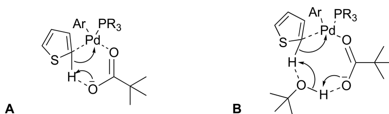
Scheme 2. (A) Carboxylate assistance C–H bond activation/cleavage in CMD transition state. (B) Proposed C–H bond activation/cleavage transition state tert -butanol assisted in CMD mechanism.
