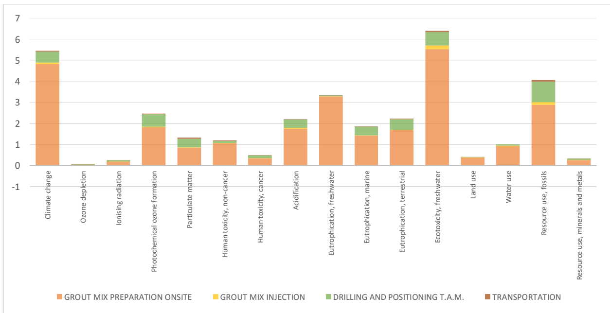
Fig. 18-3, Permeation grouting technique: impacts, normalized view.
