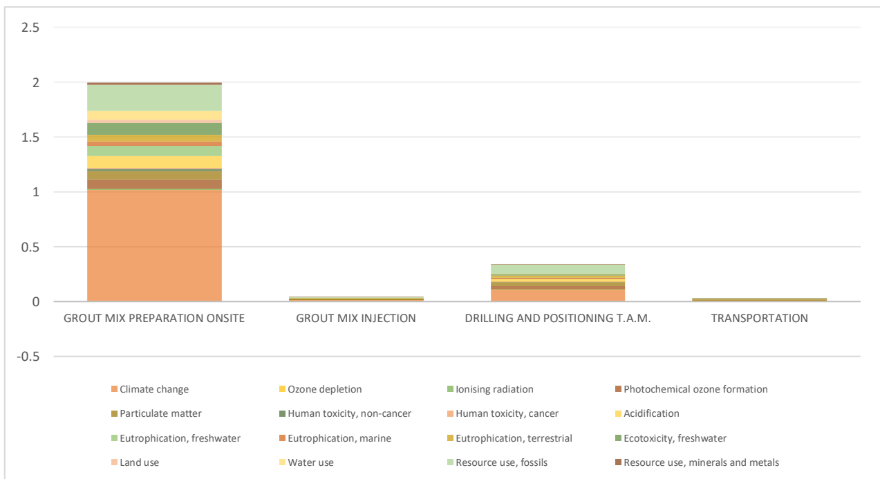
Fig. 18-5, Permeation Grouting technique: impacts, single point view.
