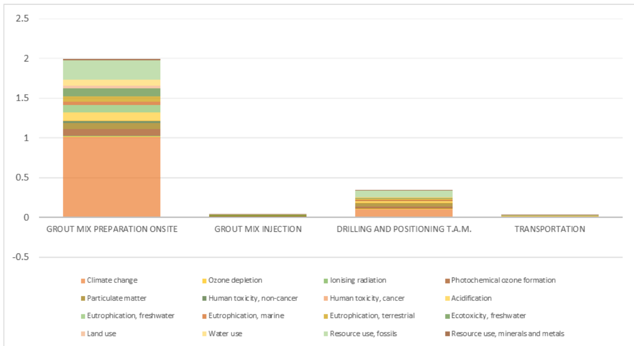
Fig. 9-16, Permeation Grouting technique: impacts, single point view.
